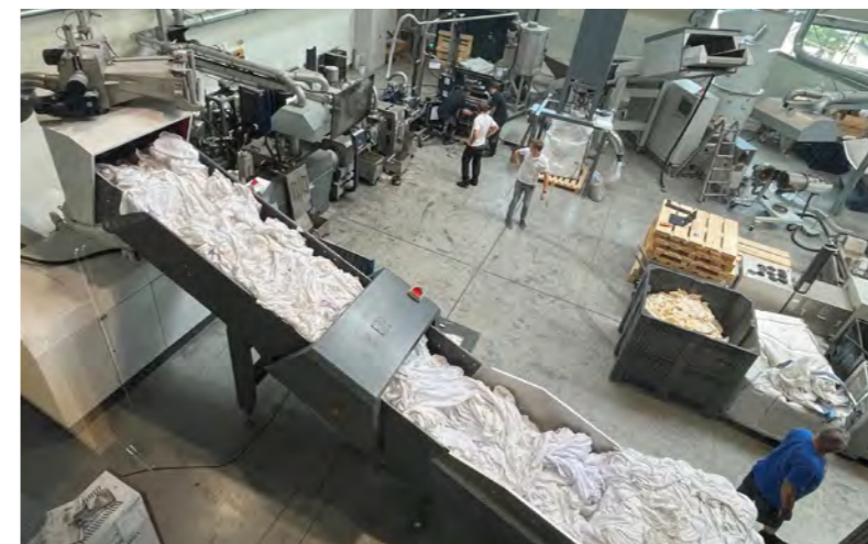
Fig. 2 Detection of metal from the uniforms before the polyester is melted into pallets
