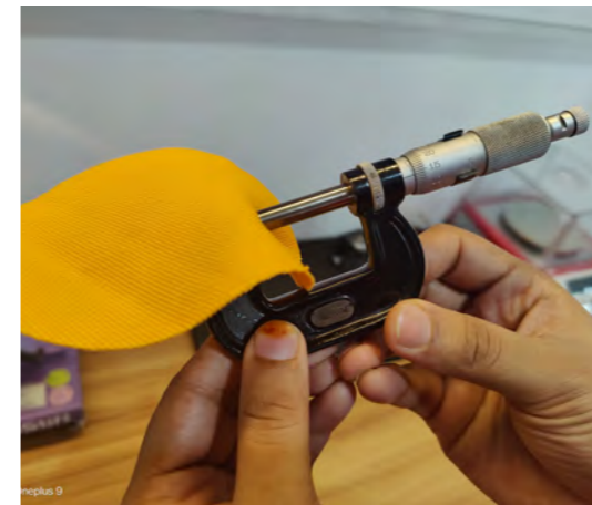
Fig. 4 Fabric testing to determine weight and density of materials for digital representation
